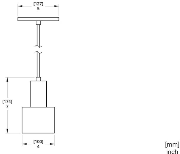
Ring is a minimalist pendant designed for clarity and comfort. Its defining feature, a large optical cutoff, hides the light source, eliminating glare and delivering illumination where it's needed most. Available in a range of beam angles, Ring is ideal for spaces that demand both performance and subtlety.
